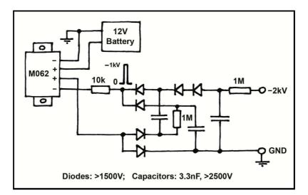
• The 1MΩ resistor at the output reduces possible electric shocks to a harmless level.
