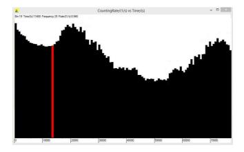
Radon concentration monitored over a period of 24 hours in a room in the basement of the building
