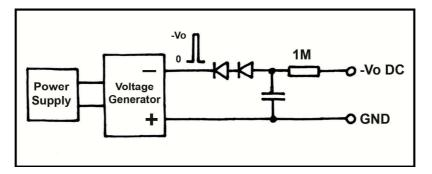
Examples of electric fence voltage generators with voltage pulses higher than 1000V:
