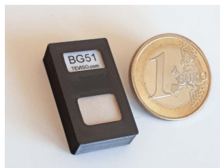
Teviso Sensor BG51 detecting alpha and beta
